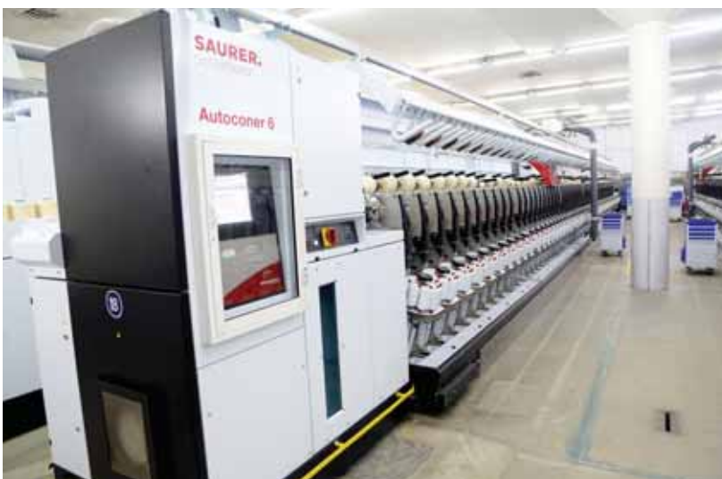
Latest Automatic Cone winding Machine Installed at our unit.
